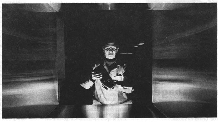
PASSING THROUGH — Ruth Bargman-Romero (1484) uses a "pass-through box" to move a mold from assembly into encapsulation, eliminating the need for gowning when transferring a product into a restricted area.
